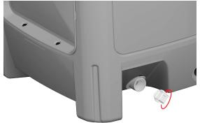
Remove Winterizing O-ring plug near the bottom of the unit. Note, there will be an initial rush of water from the unit after the plug is removed. Allow unit to completely drain, this will take 1-2 minutes. Re-install O-ring plug hand tight.
