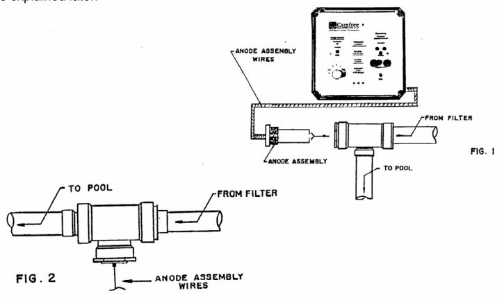
CAUTION: Figure 1 and Figure 2 are top views - looking straight down on the Ion Chamber. This is not a side view.
