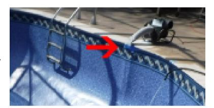
Once the water level has reached the arrows/tape line you can turn off the water and liner vacuum. DO NOT turn off any well point/ground water pumps. We will turn these pumps off when necessary. Turning these pumps off may cause structural damage to your swimming pool. The arrow in this picture can be black or blue tape instead of the red arrows.
