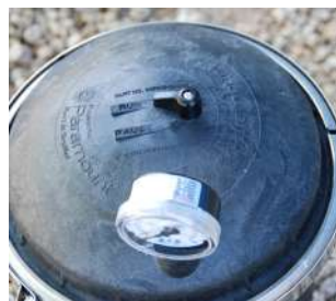
7. Turn water valve to "RUN" position
