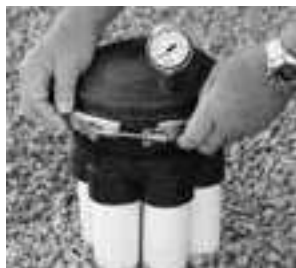
6. Place dome over module. Secure dome and base with band clamp
