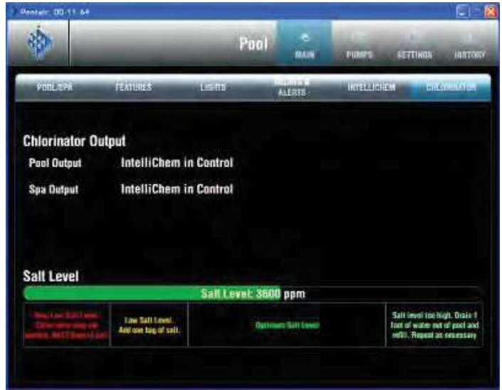
Chlorinator (IntelliChlor) with IntelliChem controller screen
